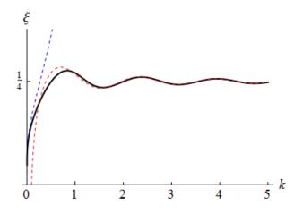
Here, the black curve is the exact formula. The red one is the Tamura formula. The blue one is the Low energy formula in the next page. The horizontal axis is the  $k = \sqrt{\lambda}$  axis
