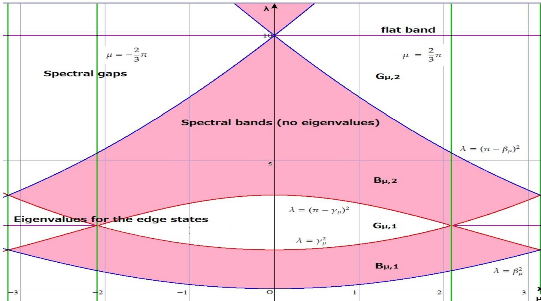
Fig. 5 The dispersion relation for  $H^\#$  in the unperturbed case.
